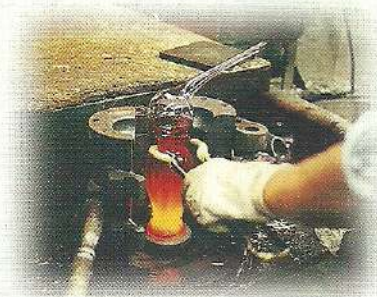
A finished piece is removed from the mould after it has been blown. The bubble on top is called the "overblow." This is scraped off and the edge is reheated before a flare or crimp is created.
