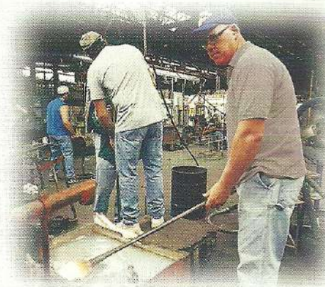
The blocker rolls a gob of molten glass in soapy water to ready the glass for the final forming mould.
