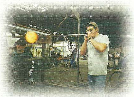
The blocker blows the first air bubble into a gob of molten glass.
