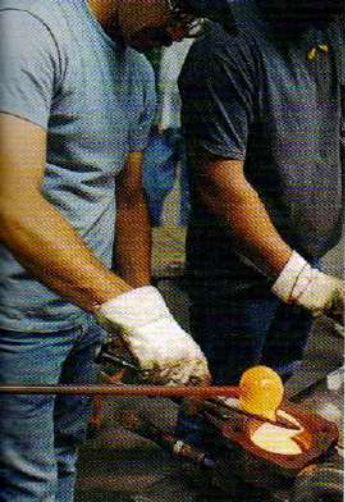
Presser Henry Holschu uses his shears to cut glass from the punty.
