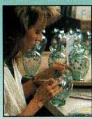
After inspection, the glass arrives at the decorating station. The chosen pattern is carefully handpainted with an oil-based paint containing finely ground glass which is then fired on for permanence. The decoration design is limited only by the size
