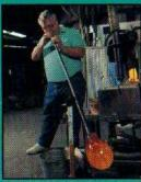
After the molten glass is gathered from the furnace, the blower shapes the initial blob into a bubble that adapts itself to the form of the mould. The exact proportions of glass in respect to the area into which it is
