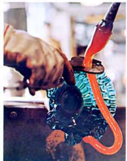
■ A molten ribbon of glass becomes a delicate basket handle. The glass is carefully shaped by hand tooling and cools into a graceful arc. All handles on Fenton Glass are attached in this same age-old manner.
