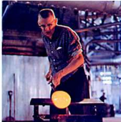
■ Shaping on the marver gives the molten glass its first crude form.
