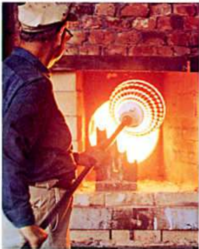
■ A long-handled "snap" holds this thumbprint bowl just before it will be "warmed-in" at the "gloryhole" to make the glass workable. Only the experienced eye of the "warming-in boy" knows when it is hot enough to be shaped into a basket by the "finisher."
