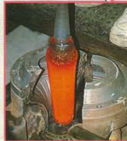
Piece being dropped in final forming mould for blowing.
